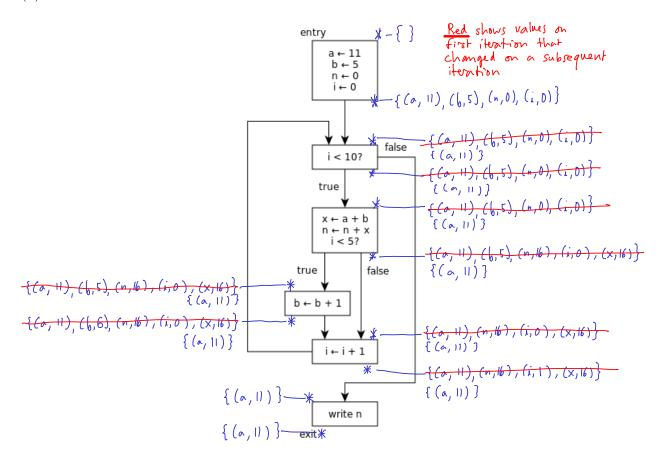
Due to the loop, the values of variables "b", "n", and "i" change, while the value of "a" remains constant.
